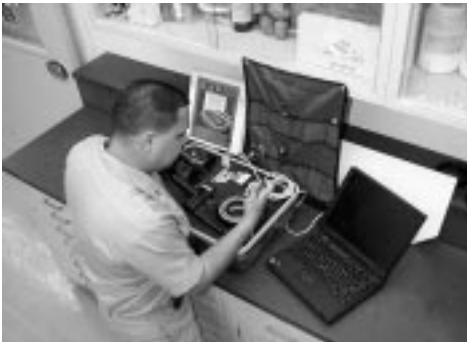
The new Ruggedized Advanced Pathogen Identification Device (RAPID) analyzer provides quick (within 30 minutes) field identification of BW agents.
